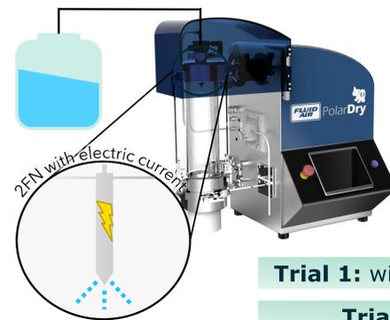
Solutions of 10% w/v of trehalose in water were prepared and spray dried using a PolarDry 0.1 (Fluid Air, France) electrostatic spray dryer, which allows to apply an electric current to its two-fluid nozzle.
