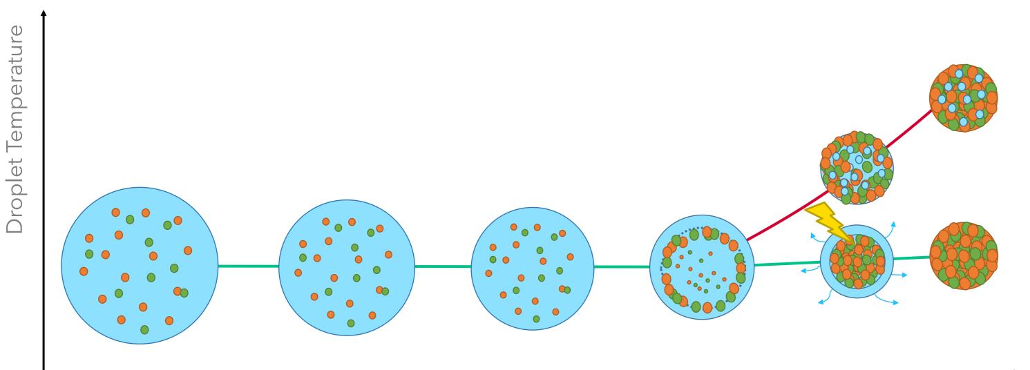
This approach has shown promising results in the past in monoclonal antibody encapsulation<sup>[3]</sup>, but its application can be extended to the manufacture of spray dried powders of thermolabile compounds for inhalation. As a proof of concept, low temperature spray drying of a trehalose solution with and without electric charge were carried out, and the differences of the products are highlighted.
